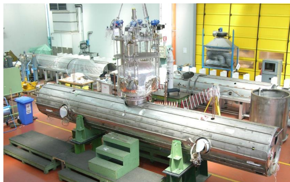
Cold mass with main He vessel and cryogenic services on top
